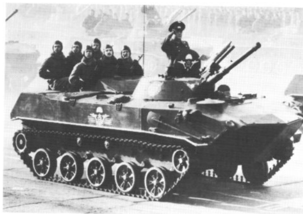
The BMD-1 Model 1973 has been the standard production version of this unique vehicle. It has the improved circular CBR air vent as compared with the square vent of the earlier Model 1970. This parading BMD is marked with the Guards insignia on the turret, and on the hull side with the badge shown as our Plate L2. (Sovfoto)
